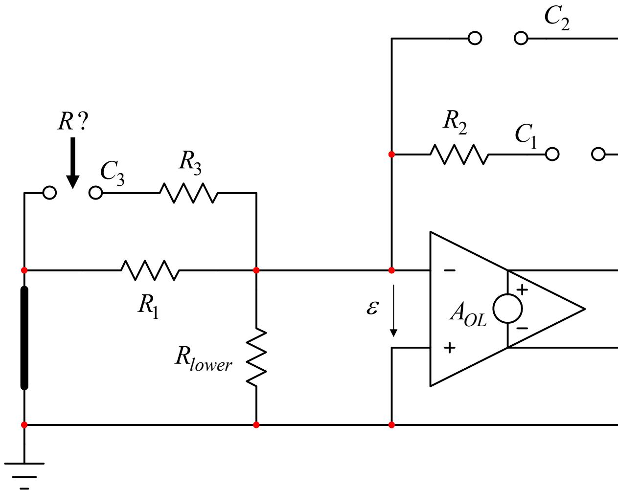
$$\tau_2 = C_2 \left( R_1 \parallel R_{lower} \right) (1 + A_{OL})$$
