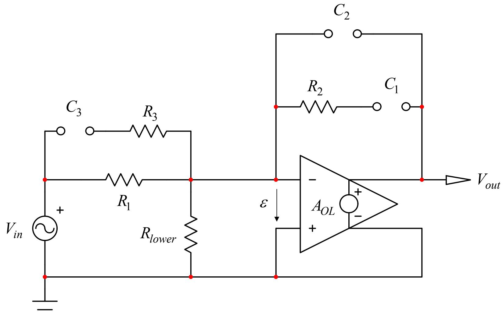
$$H_0 = -\frac{R_{lower}}{R_{lower} + R_1} A_{OL}$$
