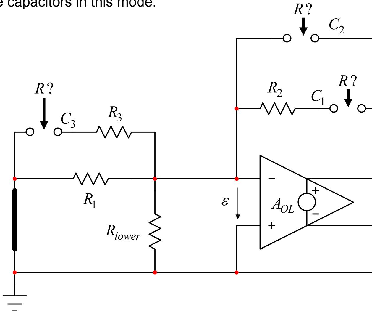
$$\tau_3 = C_3 (R_3 + R_1 \parallel R_{lower})$$
